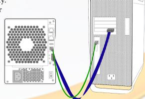
4. Flip the power switch located on the back of the RAIDBank4 to the "ON" position (labelled "-".)
